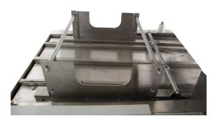
Thanks to Automatic Tray Feeding System that allows to run the machine with the single person. Just fill the storage with the trays than wait for the filled trays. Fully automated tray loading system for entrance or tray loading system onto trolley can be adapted to the machine on request. By the way system automatically fill trays, position the trays on trolleys.
